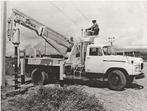
Imported into Fiji by Fiji Electricity Authority for the installation of power poles, this 3tonne crane was also the first of its kind in Fiji.
